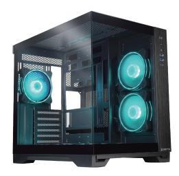
The refined internal layout supports the mounting of 360mm radiators on the top and bottom, 240mm radiators on the motherboard side, and CPU tower coolers up to 175mm in height. High-end GPUs up to 410mm can be easily accommodated, thanks to its spacious and well-ventilated configuration.
